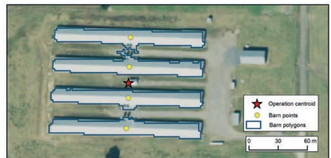
Figure 6. An example of the protocol's results - identifying polygons for individual barns, point locations for individual barns, and a single point (centroid) for the operation.
