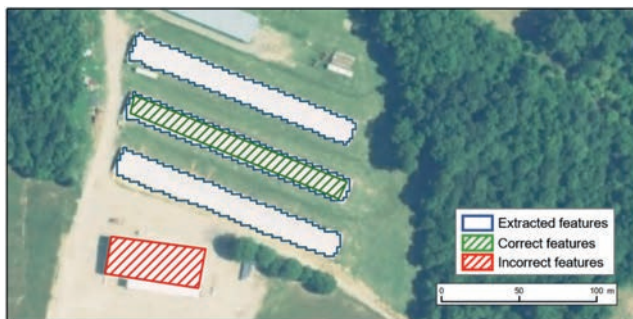
Figure 5. Correctly and incorrectly identified features were digitised to retrain the results.
