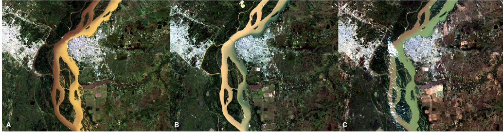
Figure 1: Natural color Landsat 8 band combinations for years 2014 (A), 2015 (B) and 2016 (C) for Corrientes city and surroundings (RGB 3,2,1).
